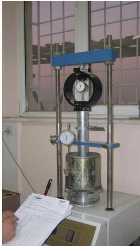
Figure 5: Reading Loads during CBR test
