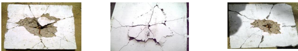
Figure 8: Failure pattern of HSC slab specimens (Al Numan & Muhammed, 2012)
